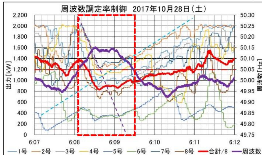
$$\text{出力低減量}[\%] = (\text{周波数} - 50.05) [\text{Hz}] \times \text{出力可能値}[\text{pu}] \times 40[\% / 0.1\text{Hz}]$$
